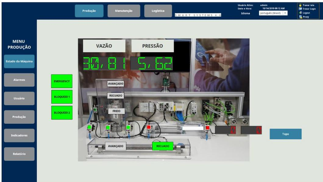
Figura 1. Tela principal do supervisório Smart System EDGE (AVENTICS, 2019).
