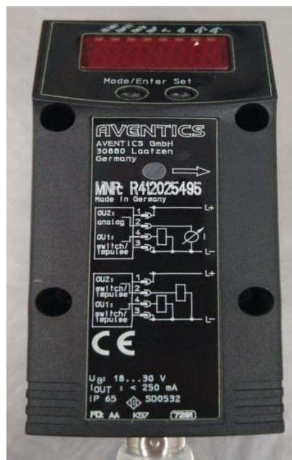
Figura 6. Frontal fluxostato Aventics (OS AUTORES).
